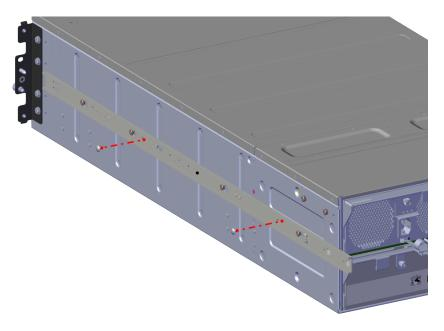
**Note:** Each side contains **3**, **M4 truss-head** screws.
