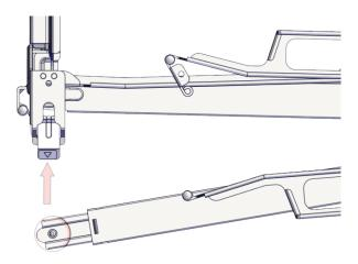
**Note:** The CMA snap location for the **Upper** arm is attached to the **Lower** CMA arm.
