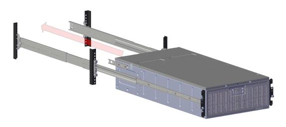
**Note:** If you are met with any resistance while completing this step, verify that the slide rails and rack mount rails are properly lined up.
