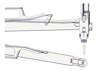
**Note:** The CMA snap location for the **Lower** arm is attached to the **Upper** CMA arm.
