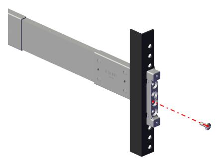
9. From the rear of the rack, attach the rack mount rail into place using one Hex flange Phillips head screw.
