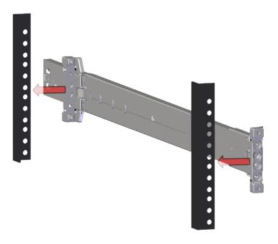
**6.** Snap the front and rear ends into the rack over the cage nuts.
