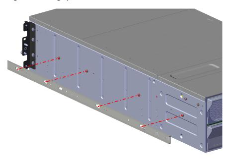
3. To lock the inner rail into place, slide the inner rail towards the rear of the chassis.
