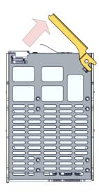
**Note:** The HDD carrier lid should open until about a 45 degree angle.
