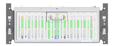
2. From the enclosure handle, pull the enclosure out until the rail kit is fully extended.
