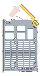
**Note:** The HDD carrier handle should open until about a 45 degree angle.
