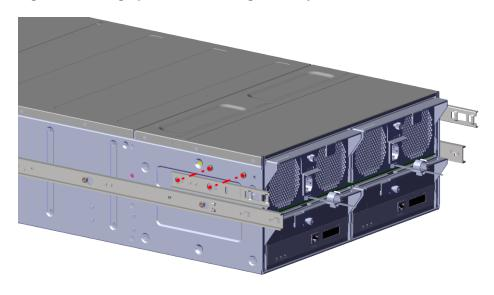
3. Press the CMA bracket into the chassis wall and slide the inner rail towards the front of the chassis.
