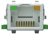
Figure 40. 10Gb RJ45 Connector LEDs
