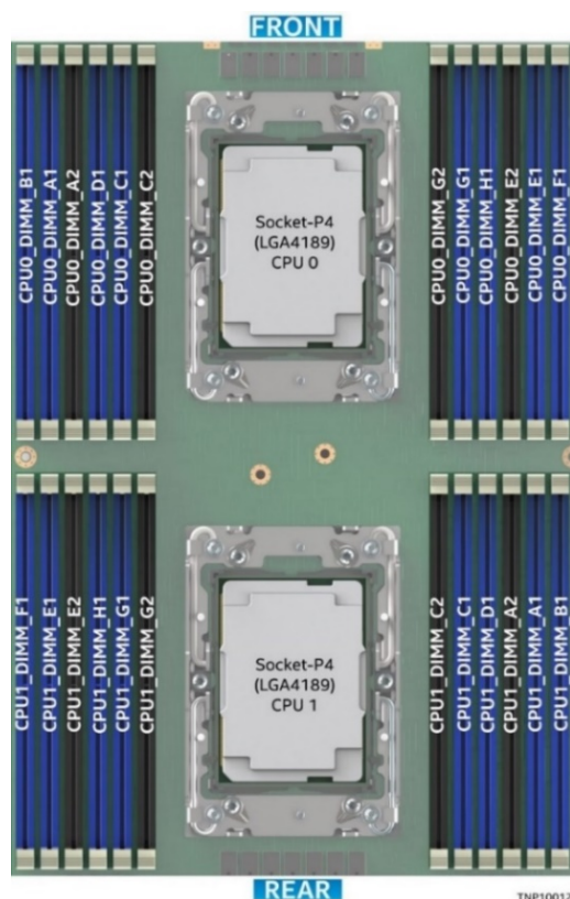
Figure 26. Intel® Server Board D40AMP Memory Slot Layout
