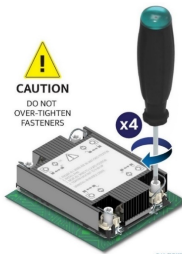
Figure 88. Tighten Heat Sink Fasteners
