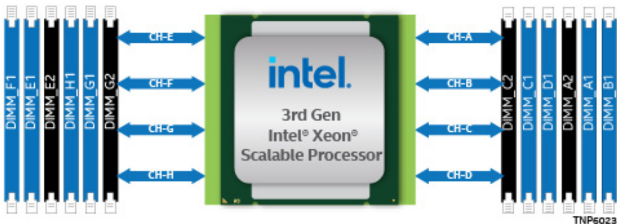
Figure 21. Memory Slot Connectivity Diagram
