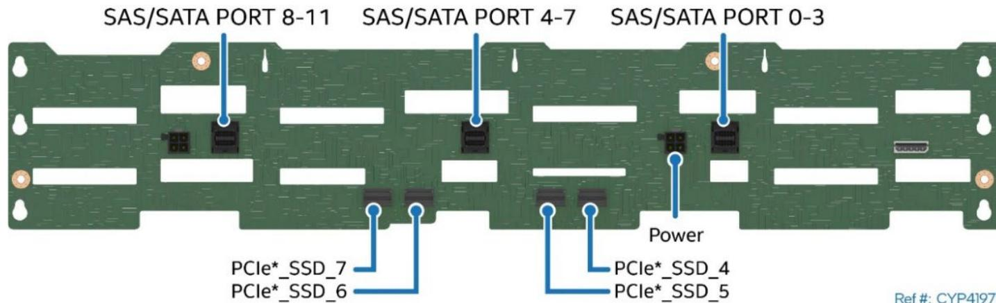
Figure 17. 2U 12 x 3.5" HSBP Connector Identification – Back Side
