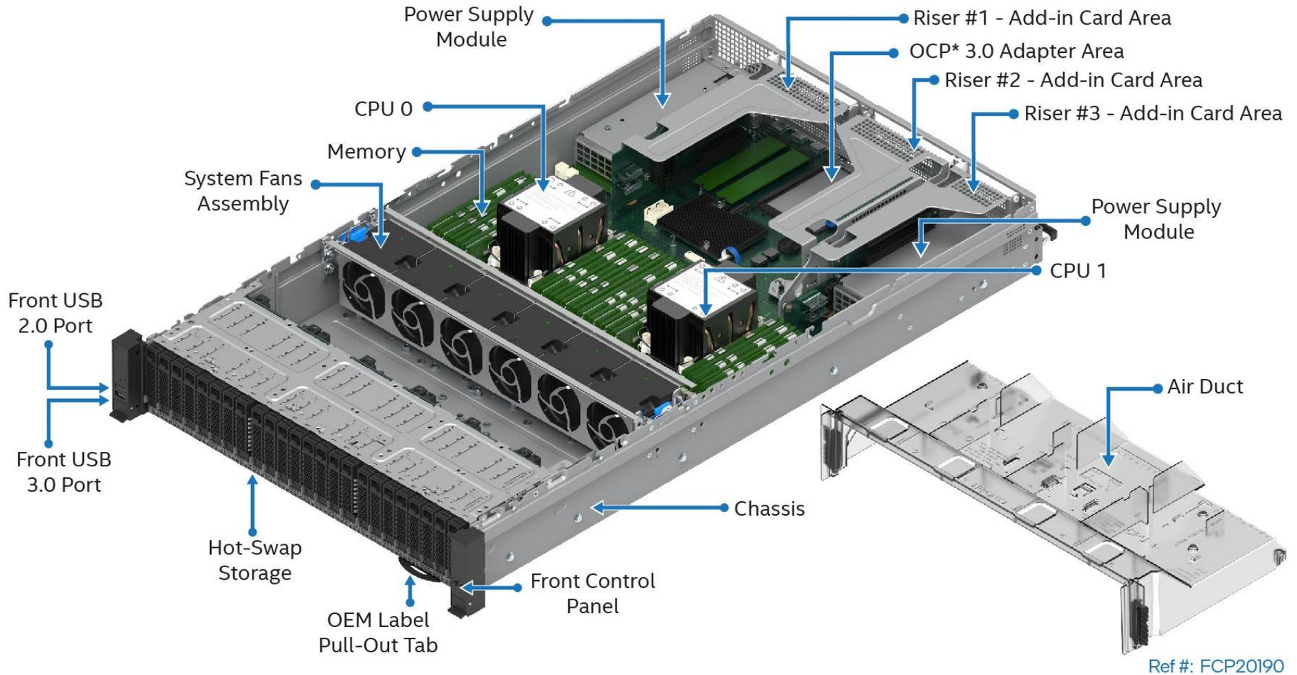
Figure 8. Intel® Server System M50FCP2UR Feature Set Identification
