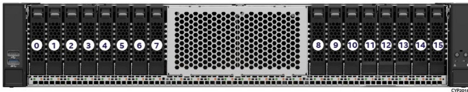
**Figure 24. 2U 16 x 2.5" Front Drive Bay Configuration**
