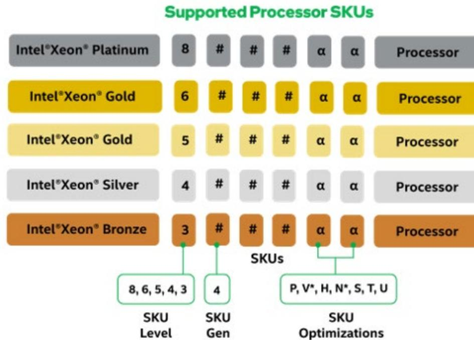
Figure 2. 4<sup>th</sup> Gen Intel® Xeon® Scalable Processor Identification
