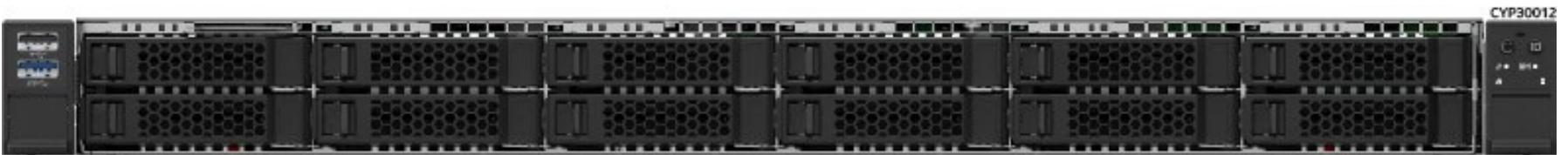
Figure 6. 12 x 2.5" Front Drive Bay Configuration – iPC M50FCP1UR212
