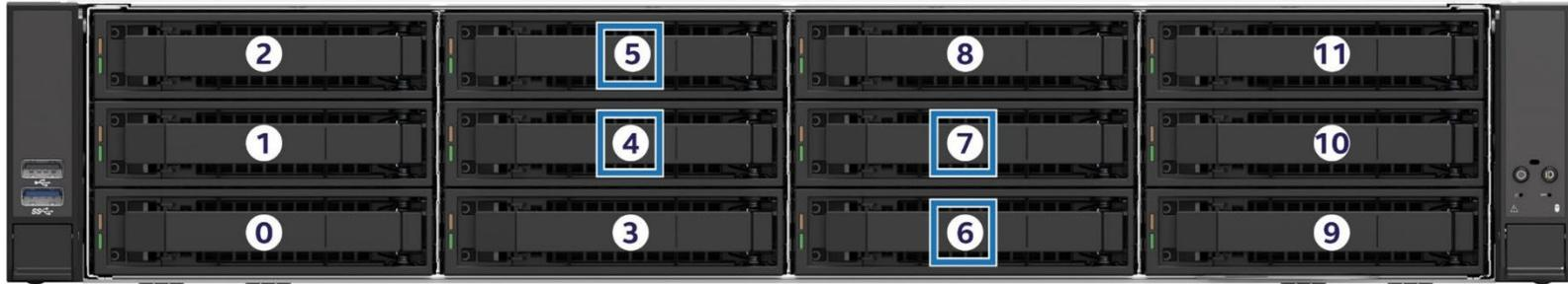
Figure 27. 2U 12 x 3.5" M50FCP2UR312 Front Drive Bay Configuration
