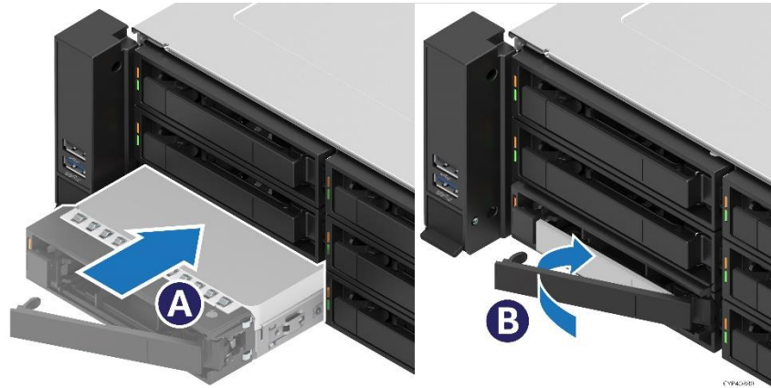
Figure 58. 3.5" Drive Carrier Installation
