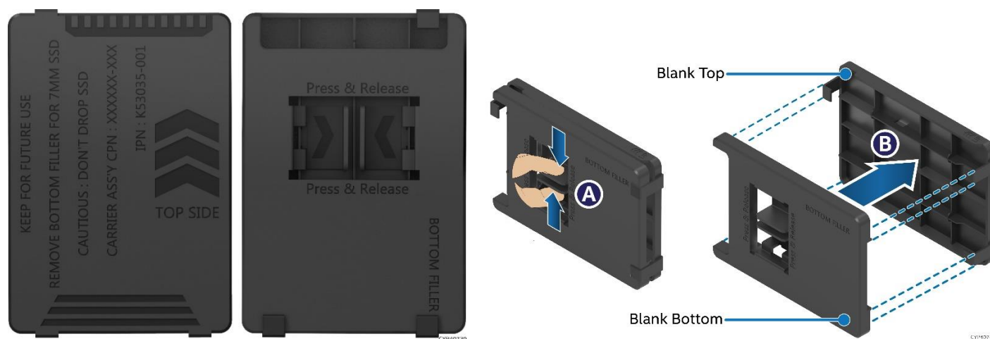
Figure 143. Separating Top and Bottom Parts of Drive Blank
