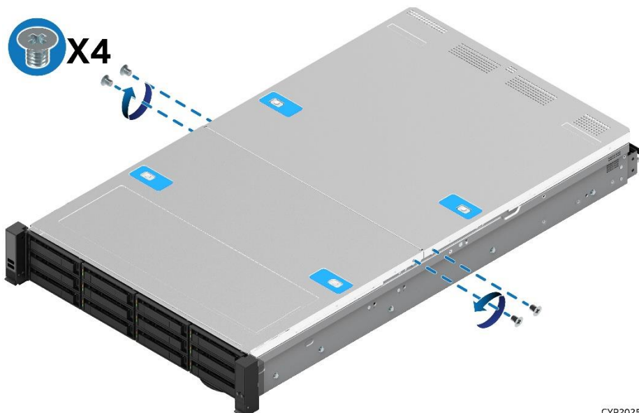
Figure 2. System Top Cover Panel Shipping Screws
