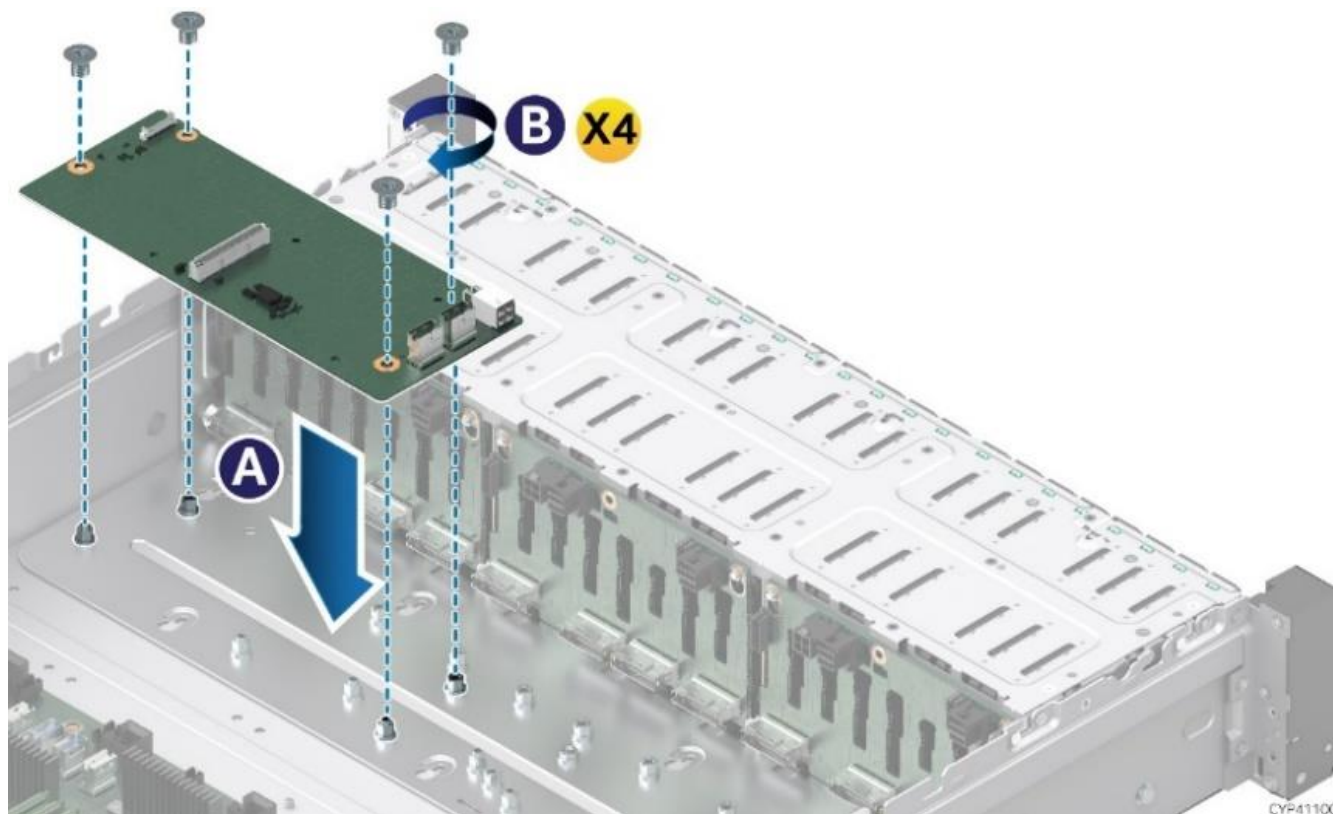
Figure 83. SAS Interposer Card Installation
