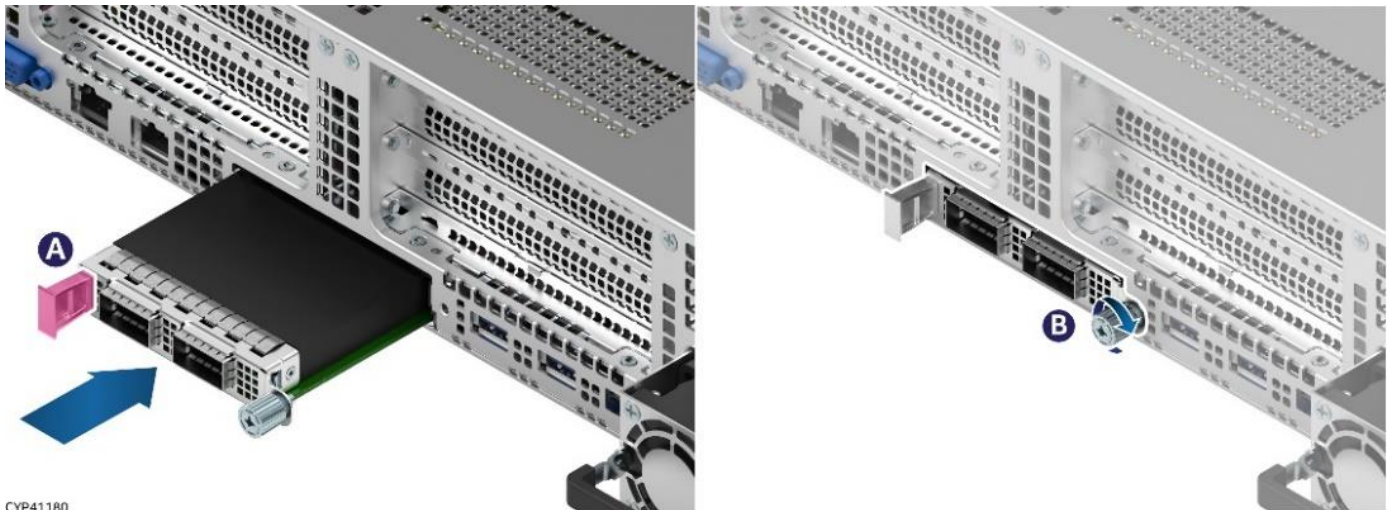
Figure 62. OCP* Adapter with Pull Tab Installation
