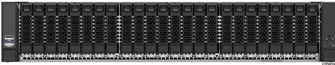
Figure 97. 24 x 2.5" Front Drive Bay Configuration
