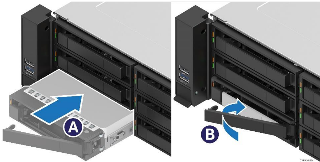
Figure 155. 3.5" drive Assembly Installation
