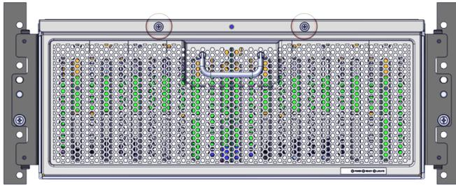
4. Turn the thumb screws counterclockwise until the cover is unsecured from the chassis.
