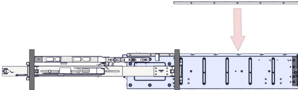
14. Slide the chassis cover towards the rear of the chassis until fully seated.
