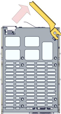
**Note:** The HDD carrier lid should open until about a 45 degree angle.
