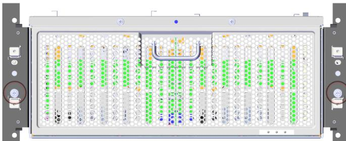
18. Verify that the thumb screws have been tightened until snug.
