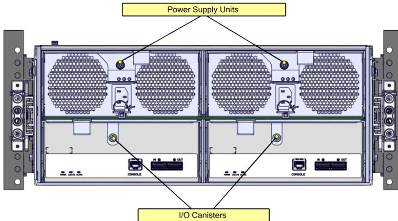
**Figure 4: Identification of Assembled Enclosure (Hard Drive Assembly)**
