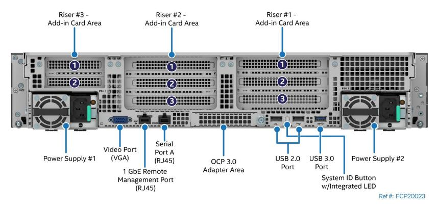
Figure 13. 2U Back Panel Feature Identification
