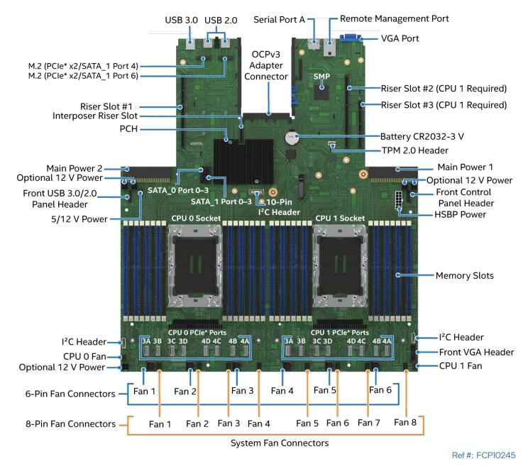
Figure 3. Intel® Server Board M50FCP2SBSTD Component / Feature Identification
