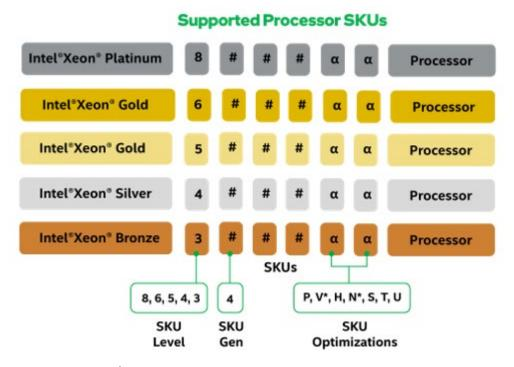
Figure 2. 4th Gen Intel® Xeon® Scalable Processor Identification
