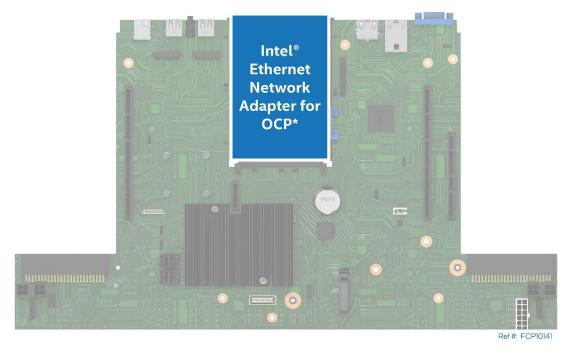
Figure 28. Intel® Ethernet Network Adapter Placement
