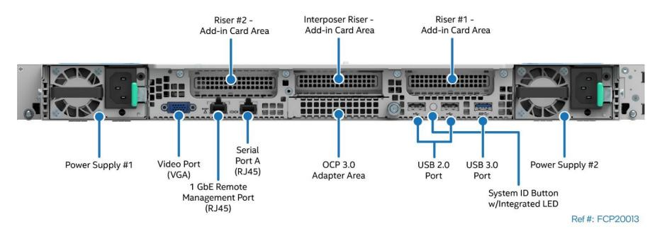
Figure 7. Back Panel Feature Identification
