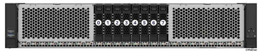
Figure 23. 2U 8 x 2.5" Front Drive Bay Configuration – M50FCP2UR208
