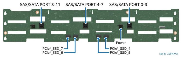
Figure 17. 2U 12 x 3.5" HSBP Connector Identification – Back Side
