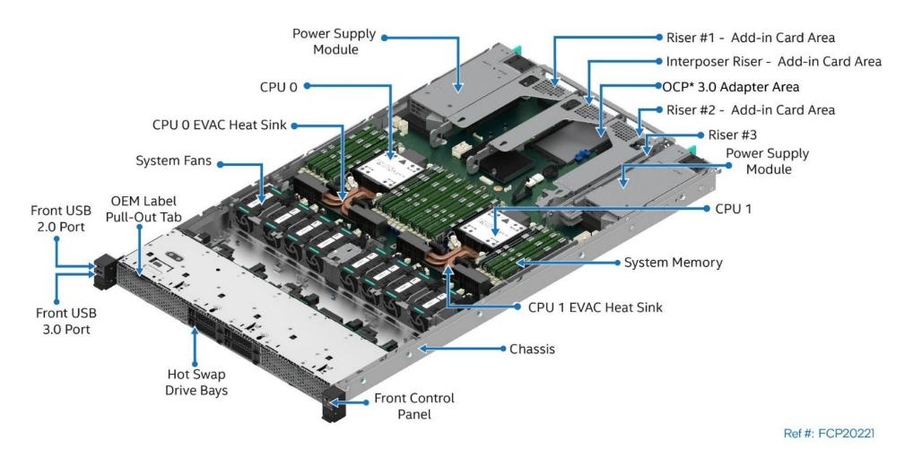
Figure 4. Intel® Server System M50FCP1UR Components Overview
