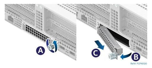
Figure 29. OCP\* Module Bay Filler Removal (2U System Shown)
