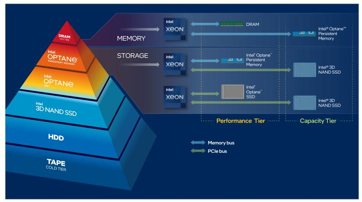
Figure 4. Intel Optane Technology creates multi-tiered memory and storage hierarchies to enable optimized workloads.
